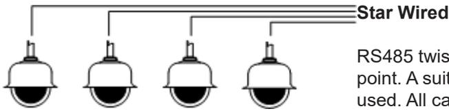
RS485 twisted pair cable is wired to each camera in a “star” from one point. A suitable RS485 star driver/data distribution product must be used. All cameras in this wiring configuration must have the RS485 (end of line) termination on.
