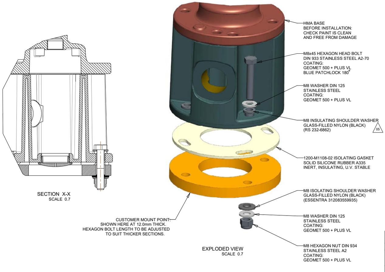
The above illustration shows how to isolate 360-Vision technology camera units from its mounting structure. A HMA version of camera mount is shown here, the same principle applies with PMA and direct mount versions.
