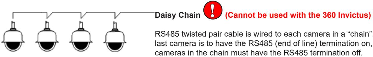
RS485 twisted pair cable is wired to each camera in a “chain”. Only the last camera is to have the RS485 (end of line) termination on, all other cameras in the chain must have the RS485 termination off.
