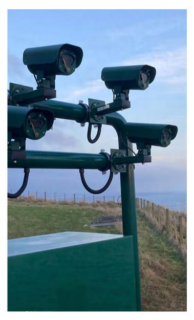
"To successfully implement the project and prevent severe corrosion, we deployed the robust 360 Vision Technology Eclipse camera, with its marine-grade stainless steel enclosure, low-power consumption, on-board recording, built-in anti-condensation heaters and self-cleaning screen wiper/washer."
