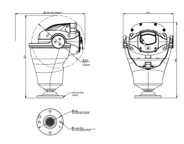
Hinged Mount Adapter with lamp Weight: 9kg
