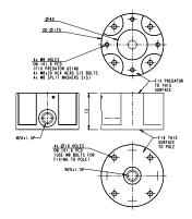
Pole Mount Bracket (PMB) Weight: 2.5kg
